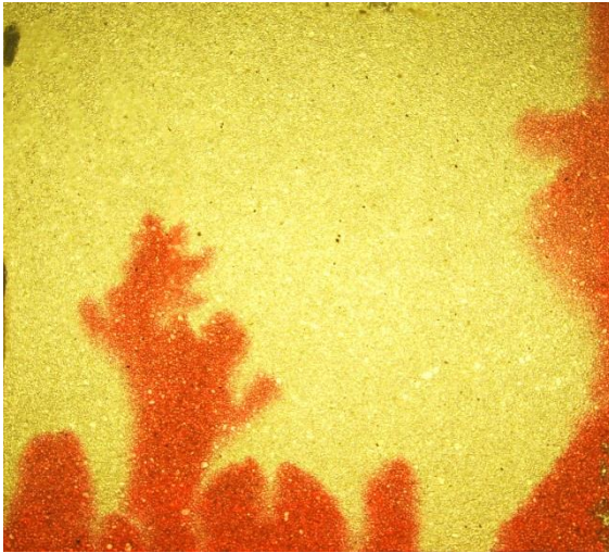
Pentane (red color) displacing mineral oil by counter-current diffusion http://www.ualberta.ca/~tayfun/eogrrc/Overview.html
